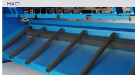
Pneumatic sheet support with automatic programmed speed; Swing movement from the plate extraction ramp.
