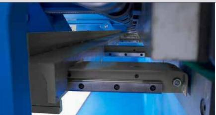
Pneumatic sheet support with automatic programmed speed;
