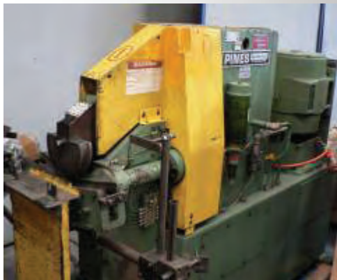
Pines 5T 32mm cap semi automatic hydraulic press bending machine
