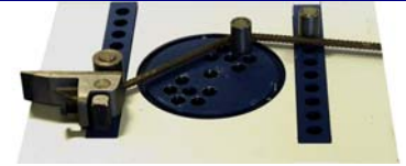
Long saddles are indispensable for double bending.
