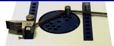
Long saddles are indispensable for double bending.
